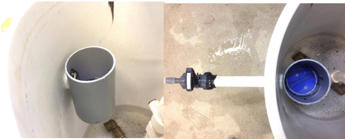
Figure 17. Weir and effluent design with section view (A) and plan view (B)
